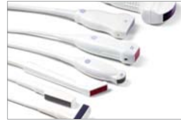
Attaching the probe allows for the LOGIQ Book XP Enhanced to auto-recognize the present application.
